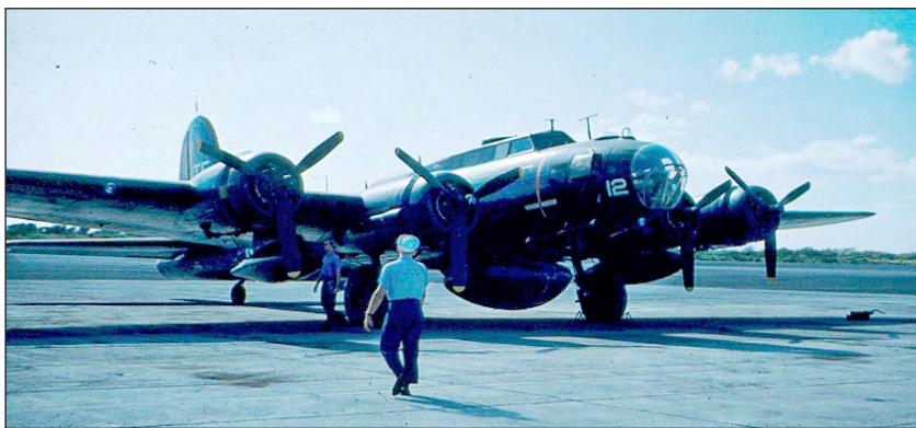
Trans-Pac PB-1W with added fuel tanks under each wing
